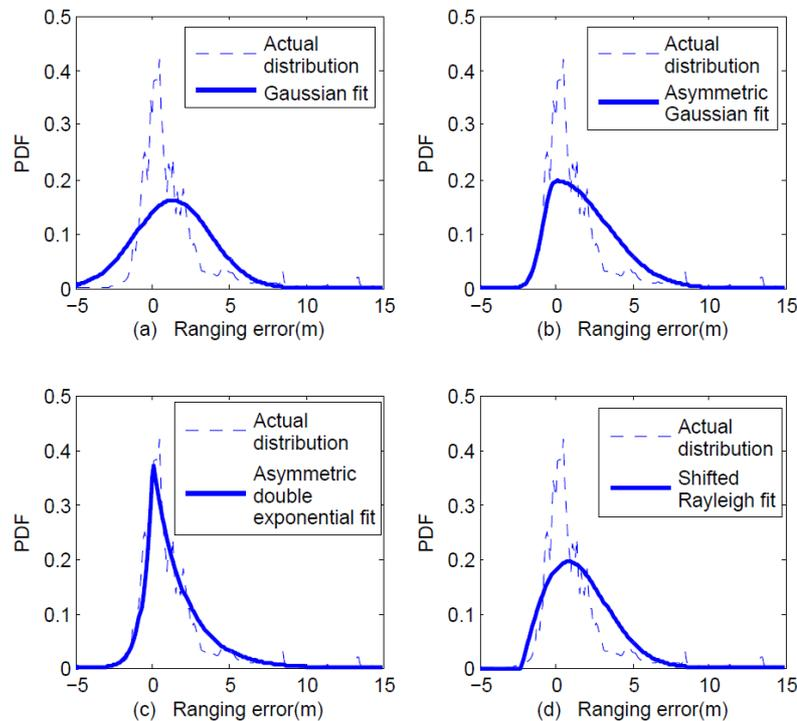
**Figure 4.** Fitting the recorded ranging error to the proposed ranging error models. (a): Gaussian model ( $\mu = 1.33, \sigma^2 = 6.08$ ); (b): Asymmetric Gaussian model ( $\sigma_P^2 = 10.46, \sigma_N^2 = 0.65$ ); (c): Asymmetric double Exponential model ( $\lambda_P = 2.03, \lambda_N = 0.60$ ); (d): Shifted Rayleigh model ( $\mu = -2.17, \sigma^2 = 9.20$ ).
