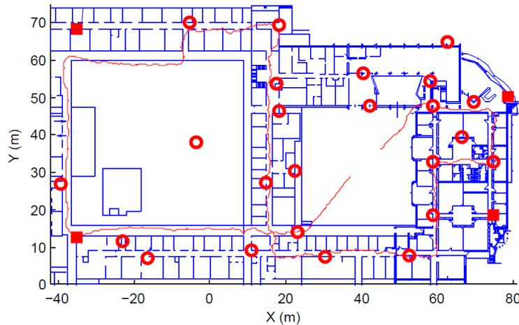
**Figure 6.** Estimated trajectory of the moving node. Red squares and red circles denote the 28 static WASP nodes, with those marked by red squares treated as anchors.
