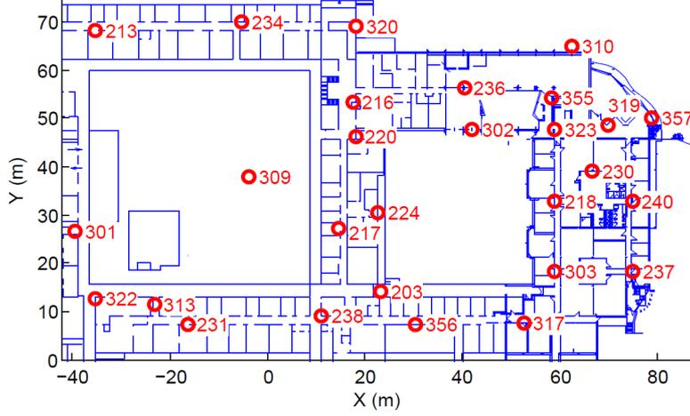
**Figure 2.** Floorplan of the deployed WASP network. The red circles denote the WASP nodes with known locations.
