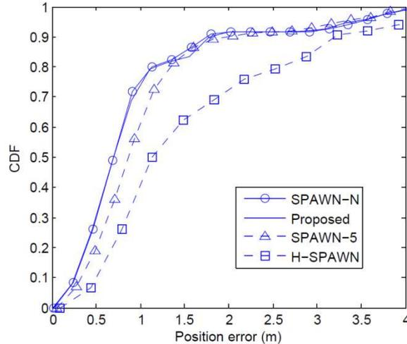
**Figure 5.** Cumulative distribution of positioning errors for static tags.
