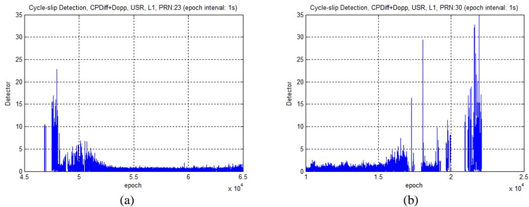
**Figure 7.** Cycle-slip Detection of Navigation grade receiver (a) PRN 23, (b) PRN 30
