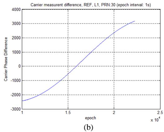
**Figure 4.** Carrier measurements difference of Survey grade receiver (a) PRN 23, (b) PRN 30
