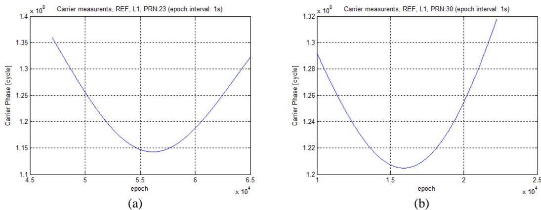
**Figure 2.** Carrier measurements of Survey grade receiver (a) PRN 23, (b) PRN 30
