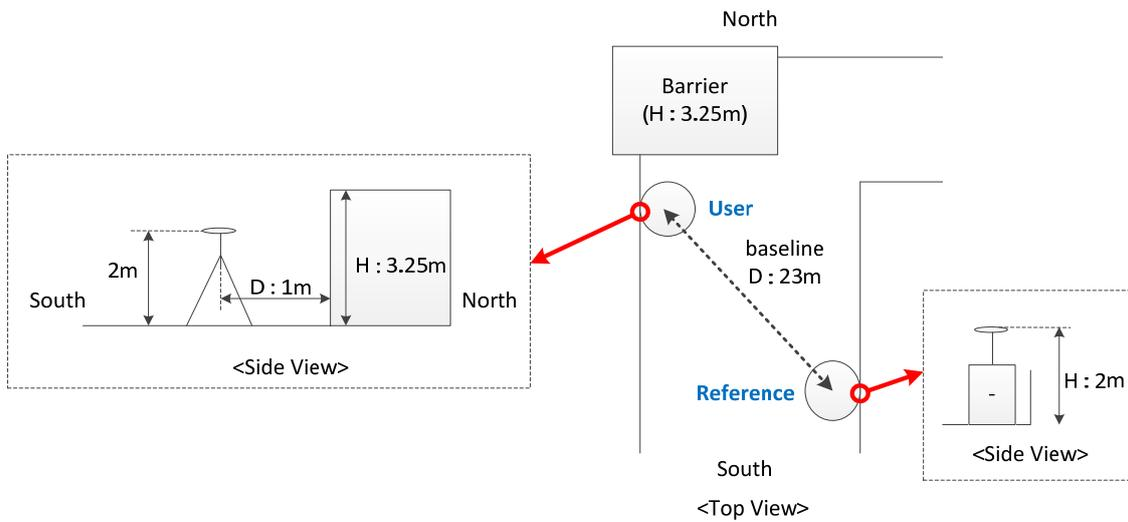
**Figure 1.** The experimental environment
